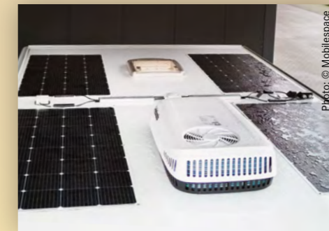
Solar panels on the trailer supplement the energy supply
