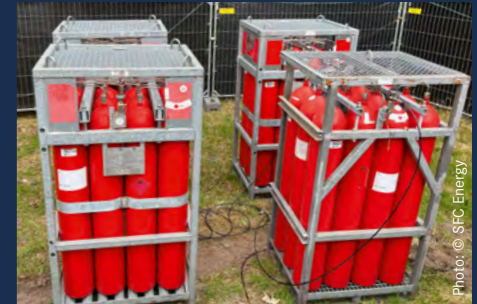
Green hydrogen, compressed at 300 bar in 50 l bottles
